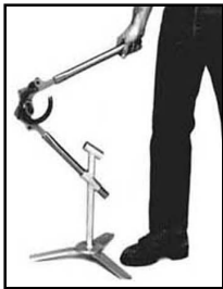
6. USE LOWER POSITION Increase leverage. Bend knees more. Good for stiff shoes.
