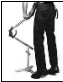
5. TWO HANDS Rise on Toe Put weight on stiff arms. Bend knees. Also good for high handle.
