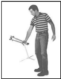
7. CARRY TOOL & STAND Grasp tool handles & top sleeve together. Carry tipped forward
