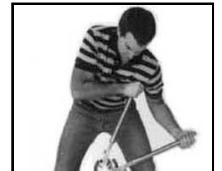
17a. SPREAD HEEL ON HOOF Position prongs on inside edge of shoe. One against heel to spread the other at opposite toe
