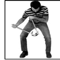
18a. CLOSE HEEL ON HOOF Position closing prongs against outside edge of shoe. One at heel to close-one at opposite toe.
