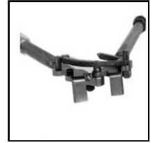
19. PREVENT SPRINGING SHOE Tilt tool when closing a heel on the hoof.
