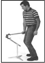
1. ONE HANDED Keep arm stiff. Don't push down with shoulder. Bend your knees and drop body.
