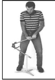
4. TWO HANDS FROM SIDE Good for high handle. Drop weight down and back
