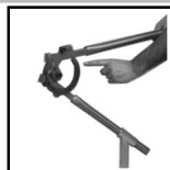
12. BENDING INTERFERENCE Avoid heel of branch from being bent hitting right shank
