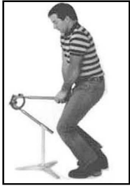
2. TWO HANDED Keep both arms stiff. If you meet resistance, bounce your weight
